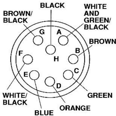
Scanner head cable connector terminals. Always route scanner head cable away from moving parts and hot steam lines. Never place close to other high voltage or high current cables which may induce harmful currents and cause malfunction.
